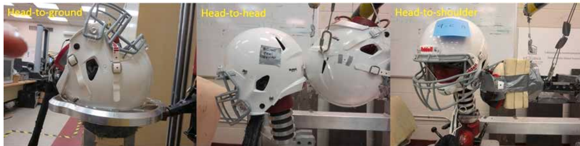
Fig. 3. Methods used for reconstructions. Left: Monorail drop rig with turf anvil for head-to-ground impacts. Center: Small NOCSAE head form and helmet as a pendulum for head-to-head impacts. Right: Pendulum with VN nitrile foam and a shoulder pad for head-to-shoulder impacts.
