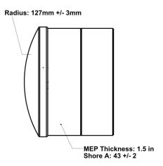
Figure 1: Pneumatic Ram Impactor Head
