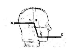
Impact Area – for a headgear that is to be tested on the medium headform\*, the impact area must include all locations on the headform which lie on or above a line (AB) 1  $^3$ /16 inches above and parallel to the BASIC PLANE posterior to the CORONAL PLANE and on or above a line (CD) 2  $^3$ /8 inches below and parallel to the BASIC PLANE forward of a point 1  $^3$ /16 inches anterior to the CORONAL PLANE, and forward and above line (BC) which connects these two lines.
